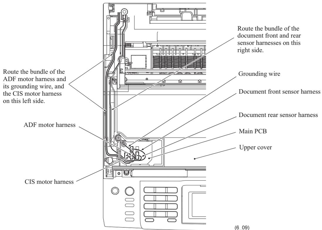
**Routing B: Document front and rear sensor harnesses on the ADF unit (for models with ADF)**
