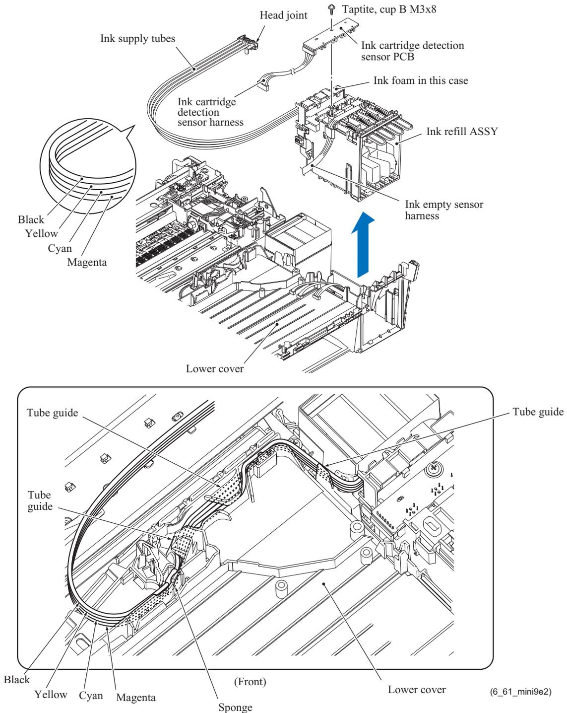
**Assembling Note:** After mounting the ink refill ASSY, route the ink supply tubes on the lower cover, aligning the four colors in the order as shown above.
