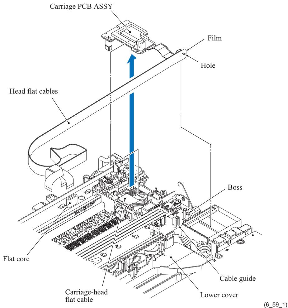
**Assembling Note:** When mounting the carriage PCB ASSY, route the head flat cables, observing instructions given on the next page.
