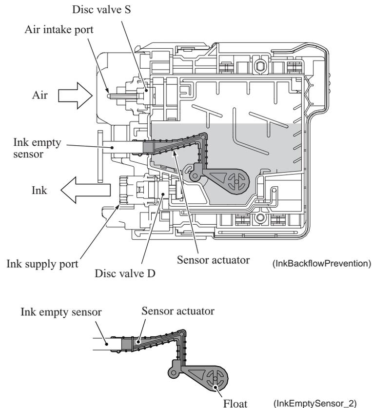
Attached to one end of the sensor actuator is a float. When there is ink in the cartridge, buoyancy lifts the float, rotating the sensor actuator about a pivot near the center of the actuator to block the light beam to the ink empty sensor, indicating that there is ink.
