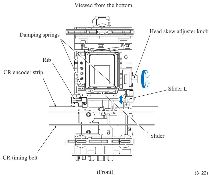
**Height adjustment of the head/carriage unit**
