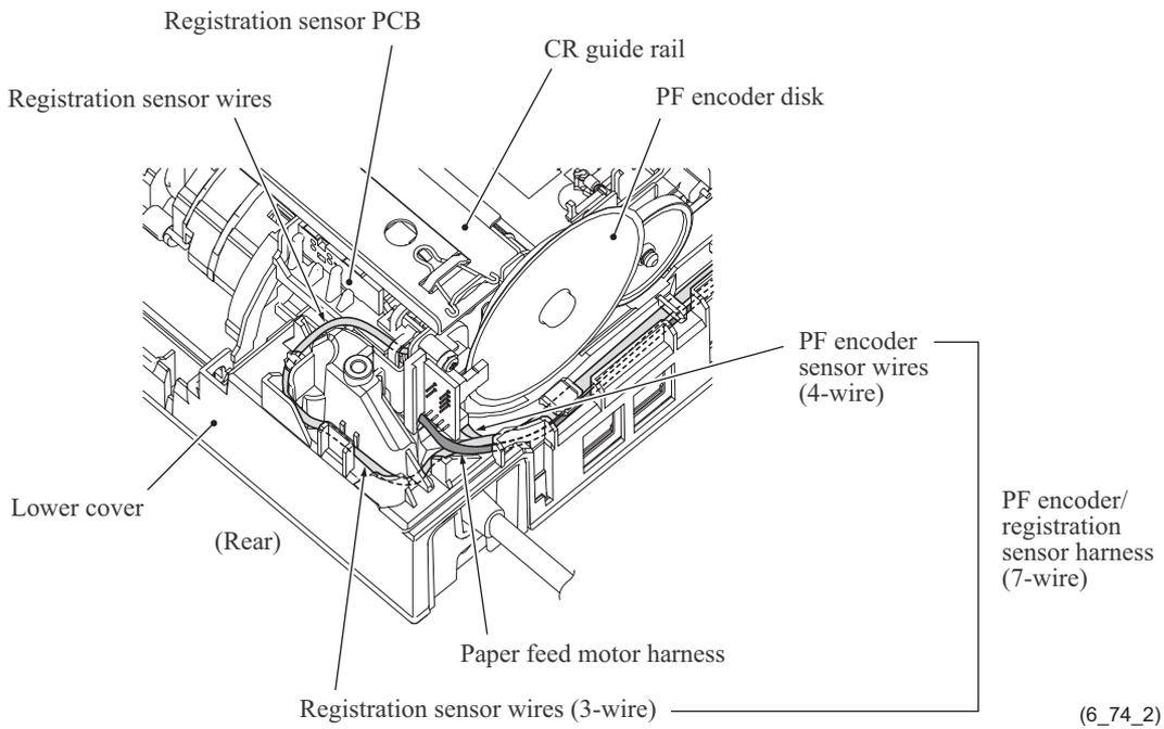
**Routing L: Harnesses, flat cables and ink tubes on the lower cover**
