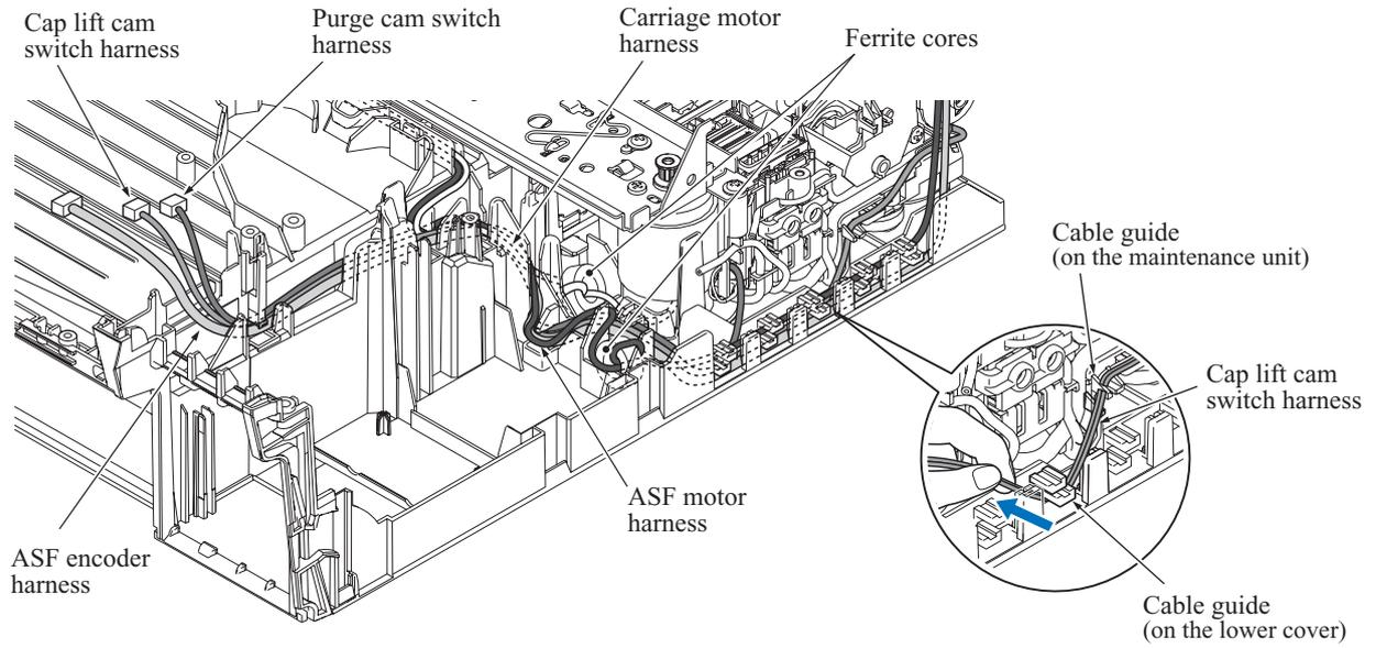
**Note: When routing the cap lift cam switch harness on the lower cover, pass it under the 3rd cable guide counted from the rear without any slack, pulling it with your fingers.**
