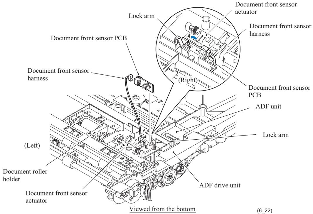
**Assembling Note:** Route the document front sensor harness through the cable guides provided on the ADF unit as shown below. Also route the ADF motor harness through the cable guides together with the document front sensor harness.
