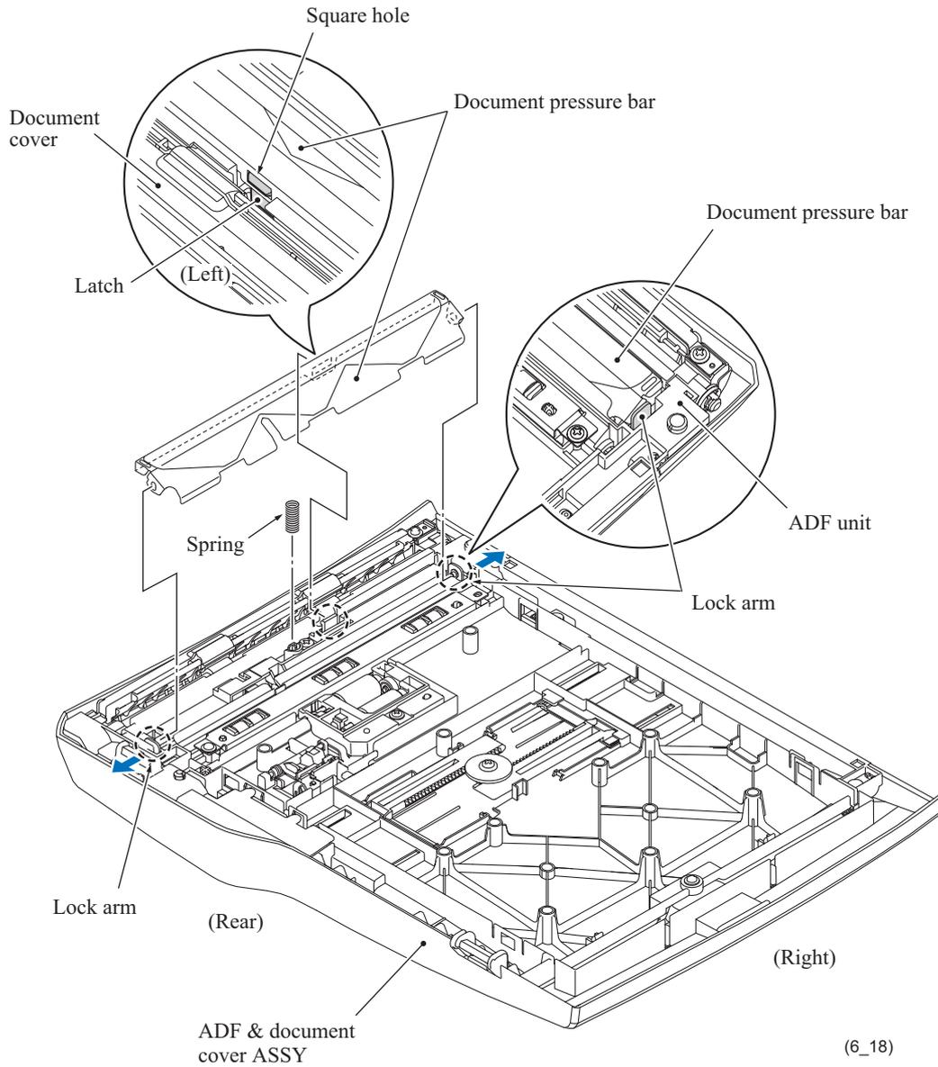
**Assembling Note:** When handling the document pressure bar, be careful not to stain or scratch the white reference film on the bar.
