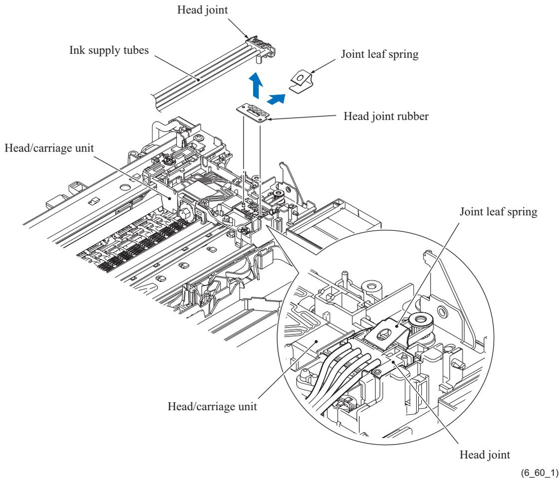
**Assembling Note:** Before setting the head joint, make sure that the head joint rubber is set on the head/carriage unit as shown above. Then secure the head joint to the head/carriage unit with the joint leaf spring.
