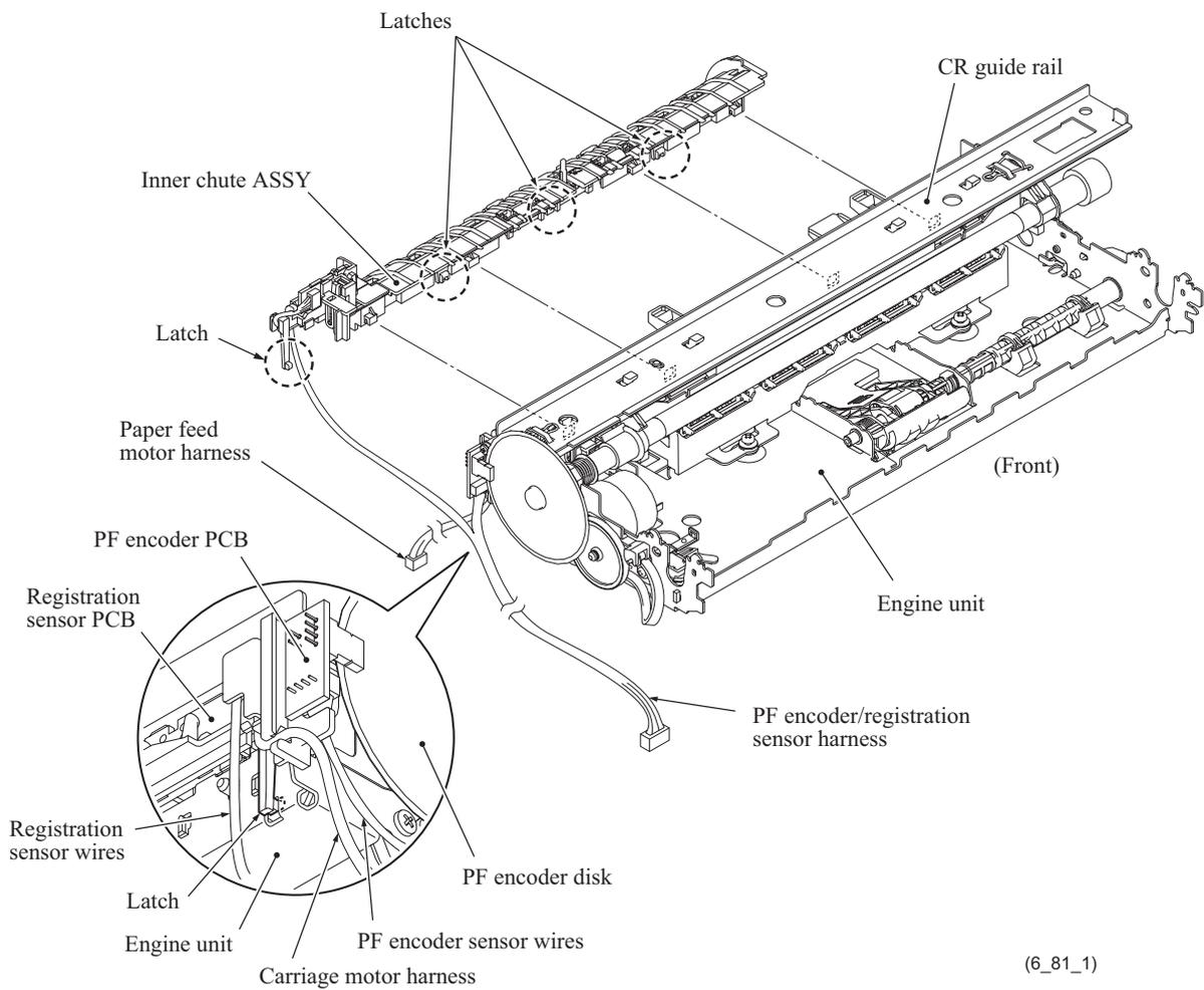
(18) Turn the registration sensor actuator in the direction of the arrow shown below and take it off the inner chute ASSY. The sensor actuator spring comes off.
