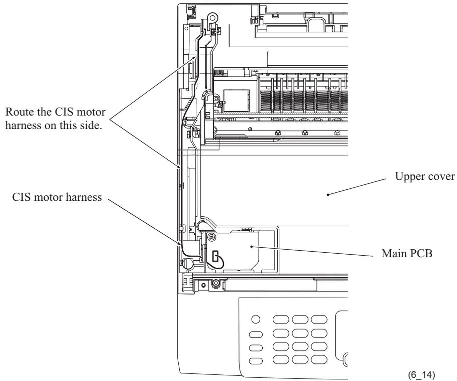
**Models with ADF:** Route the document front and rear sensor harnesses, CIS motor harness, ADF motor harness and grounding wire as shown below.
