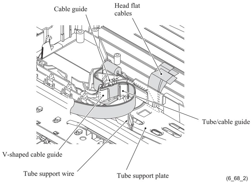
**Routing J: Purge cam switch harness, cap lift cam switch harness, carriage motor harness, and ASF motor/encoder harness on the lower cover**
