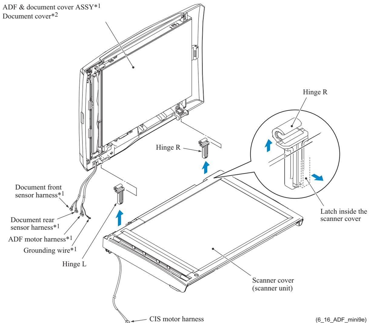
**Assembling Note:** When mounting the ADF & document cover ASSY\*1 on the scanner cover, put a magazine or a stack of paper about 2 to 3 cm (one inch) thick between them to secure room for looseness of harnesses. Do not use the one that may scratch or contaminate the scanner glass.
