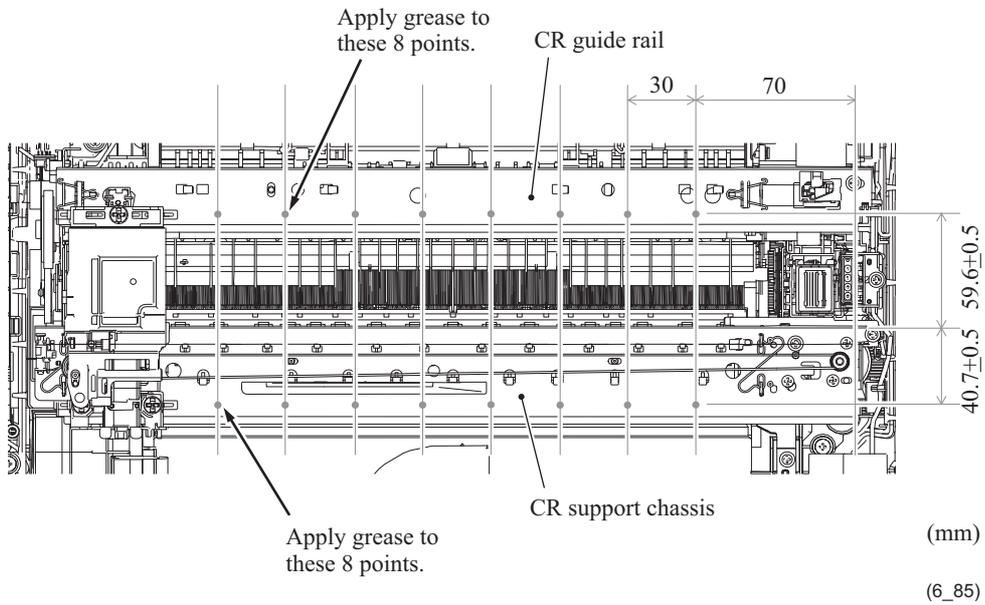
■ **CR support chassis (front and rear sides of upright rear edge)**
