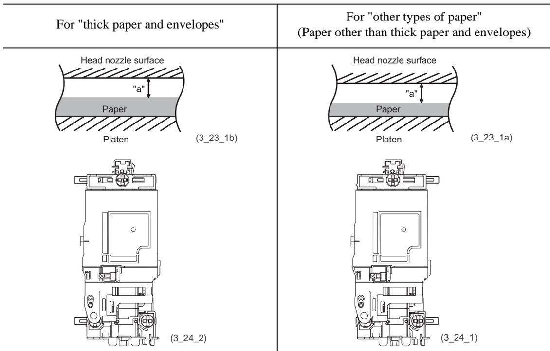
As listed below, the printer driver on the connected PC or the paper type setting on the machine controls the slider cams to determine the height of the head/carriage unit.
