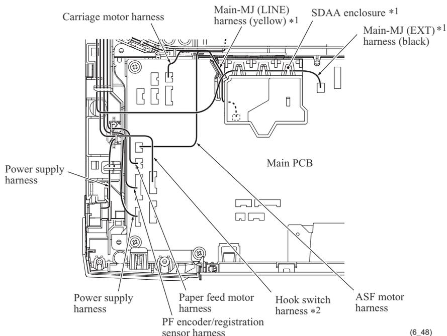
(3) **For MFC:** Release the main-MJ (EXT) harness from the cable guides provided on the SDAA enclosure. Press the right and left ends of the SDAA enclosure inwards and remove it from the main PCB. Then disconnect the main-MJ (LINE) harness (2-wire, yellow) from the main PCB.
