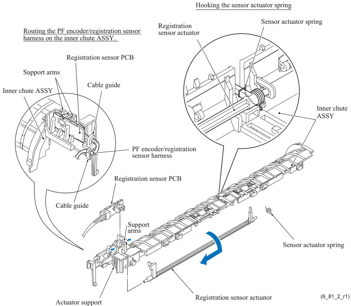
(20) At the left end of the engine unit, remove the screw that secures the PF encoder PCB and its support to the engine unit, taking care not to touch the PF encoder disk (if it has not been removed in [Section 6.1.13](#)). Then remove the PF encoder PCB and its support to completely release the PF encoder/registration sensor harness unit.
