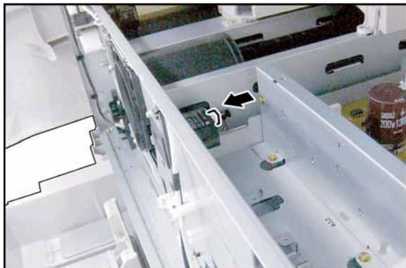
(19) Connect the **MC Harness** to the Mechanical Counter.
