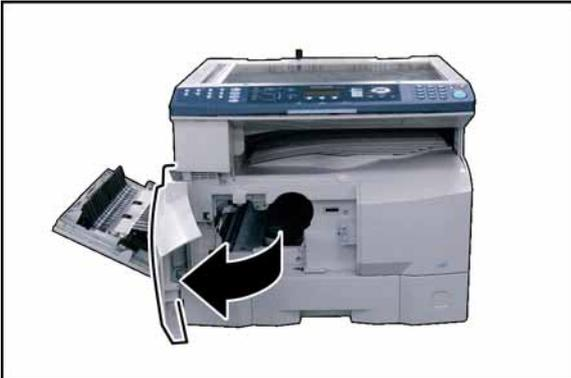
**<Installing the Process Unit>**
